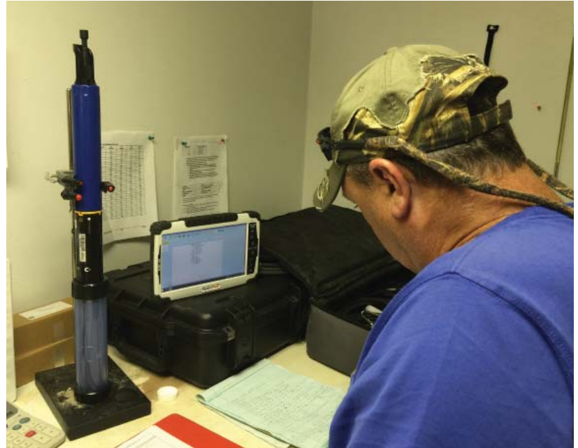
Calibration of the multiprobe sonde
