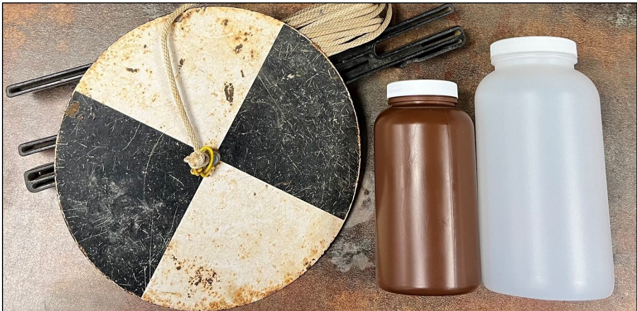
A SECCHI DISK, CHLOROPHYLL-A SAMPLE BOTTLE, AND A TOTAL PHOSPHOROUS SAMPLE BOTTLE
